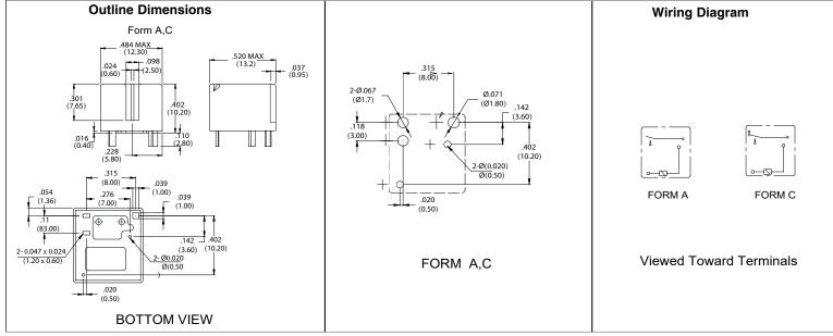
Dimensions in inches with millimeters in brackets below. Tolerance: ± .010"
