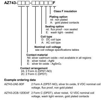
AZ743-2AE-230AF 2 Form A (DPST-NO), silver tin oxide, 230 VAC coil voltage, flux proof, non gold plated
