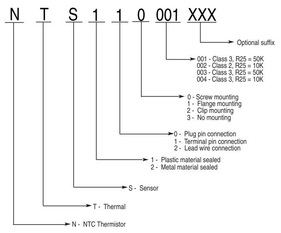
Zettler NTS Thermistor sensor is designed according to UL 1434 or customer custom requirements. All components have excellent reliability and are RoHS compliant. Precision range term 1%, 2%, 3%, or 5%.
