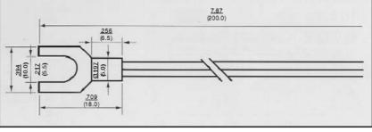
Combined housing sealed temperature sensor is normally housed by metal and plastic material together. It has the advantage of plastic housing sealed and metal housing sealed sensors, quick thermal response, strong construction, easy to have complex shape, easy to fasten, etc. to +250°C environment.
