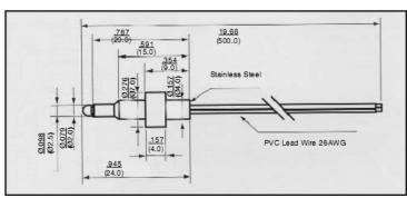
Simple housing packaged temperature sensor, the NTC normally is packaged by Teflon or PVC heat shrink sleeve or sealed by epoxy. This kind of sensor has simple construction, is economical and has good thermal response. They normally can be used in a clean application environment without strict environment conditions.
