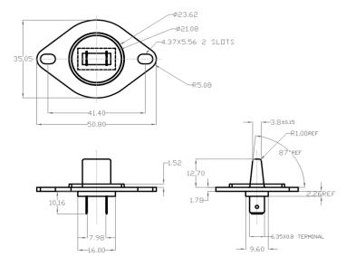
The NTC can be sealed completely in a plastic housing or can be exposed, this will be determined by customer's applications thermal response and dielectric strength requirement.
