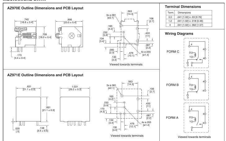
Dimensions in inches with metric equivalents in parentheses. Tolerance:  $\pm 0.010$ "
